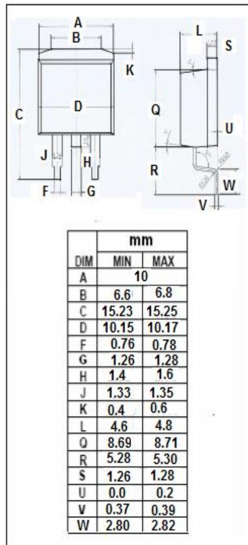
**Isc N-Channel MOSFET Transistor****RU75230S****ELECTRICAL CHARACTERISTICS** $T_c=25^\circ\text{C}$  unless otherwise specified
