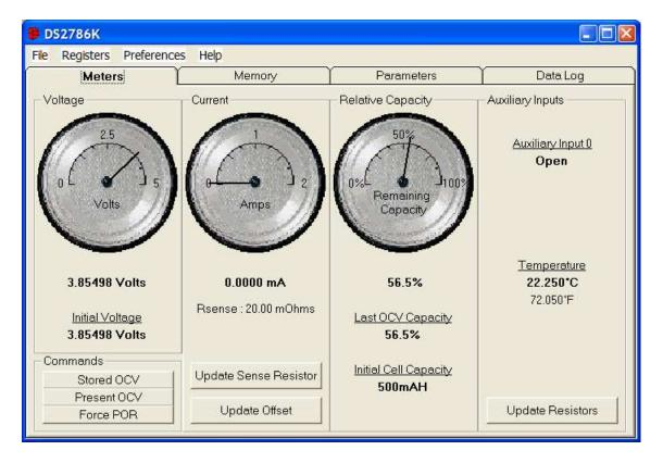
The Meters Tab displays the latest real-time measurements of cell voltage, auxiliary inputs, temperature, current and relative capacity with both analog meter readouts and digital values.
