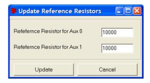
A known 10K resistor is used to determine the resistance of the Auxiliary Inputs. If the values of the resistors are not exactly 10K, or if other values are desired for the known resistors, simply left-click on the Update Resistors button and the Update Reference Resistors window will appear. Simply enter the correct reference resistance and left-click Update. Once again, this is only a software value, so it is not stored on the device, but it will be recalled each time the program is started.
