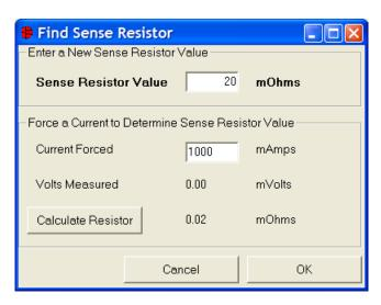
The sense resistor value used to calculate the current reading is shown in the current section. Left-click on the Update Sense Resistor button to open the Find Sense Resistor window.
