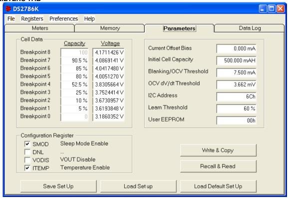
The Parameters Tab gives the user access to the entire Parameter EEPROM memory. The DS2786 comes preloaded with a best fit curve that was calculated based on characterization data taken from cells of various sizes and manufacturers. To change any of this information, simply click on the desired text field and enter the new value.
