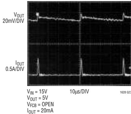
**Constant Frequency (Burst Inhibit) Operation (Figure 13)**
