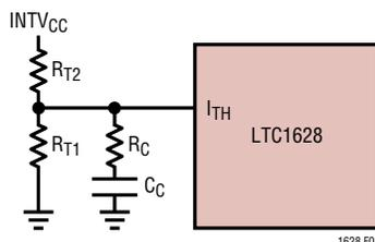
**Figure 8. Active Voltage Positioning Applied to the LTC1628**
