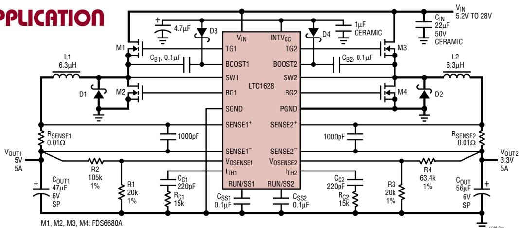
Figure 1. High Efficiency Dual 5V/3.3V Step-Down Converter
