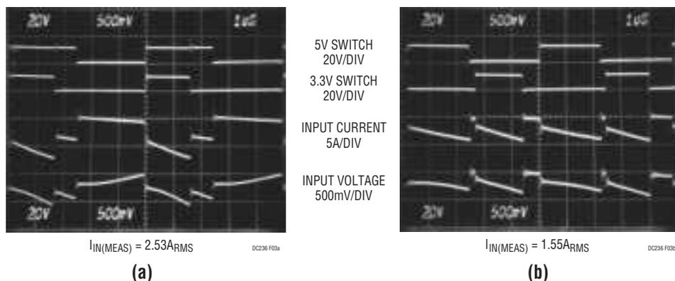
**Figure 3. Input Waveforms Comparing Single-Phase (a) and 2-Phase (b) Operation for Dual Switching Regulators Converting 12V to 5V and 3.3V at 3A Each. The Reduced Input Ripple with the LTC1628 2-Phase Regulator Allows Less Expensive Input Capacitors, Reduces Shielding Requirements for EMI and Improves Efficiency**
