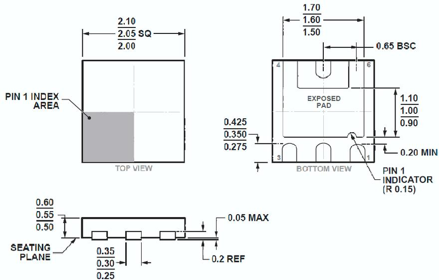
Figure 14. 6-Lead Lead Frame Chip Scale Package [LF CSP\_UD]
