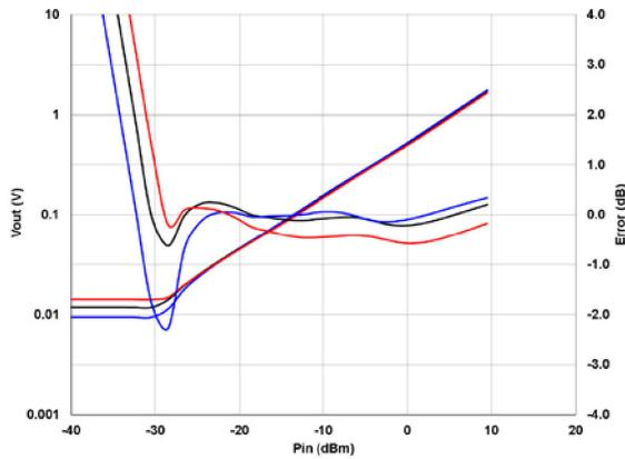
Figure 11  $V_{OUT}$  and Conformance Error vs.  $P_{in}$  and Temperature at 40GHz (Data Truncated by Measurement Setup).
