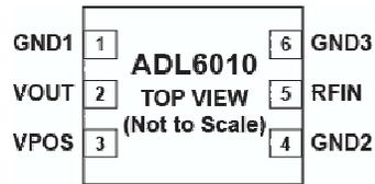
Figure 2. Pin Configuration
