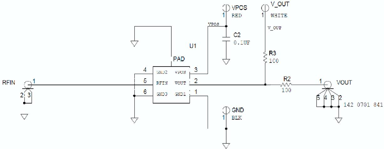
Figure 13 ADL6010 Evaluation Board Schematics
