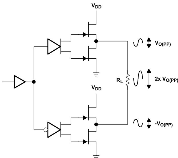
**Figure 23. Bridge-Tied Load Configuration**
