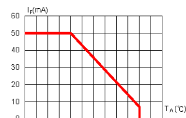
Fig.4 Allowable Forward Current vs. Ambient Temperature
