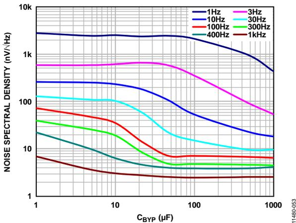
Figure 53. Noise Spectral Density vs. C<sub>BYP</sub> for Different Frequencies
