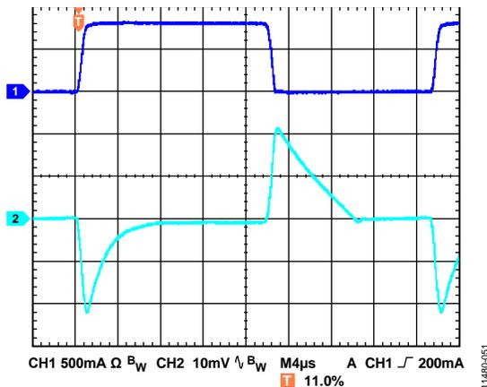
Figure 51. Output Transient Response,  $V_{OUT} = 5\text{ V}$ ,  $C_{OUT} = 10\ \mu\text{F}$
