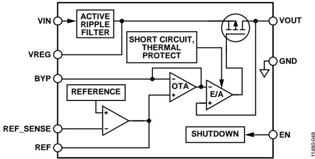
Figure 48. Adjustable Output Voltage Internal Block Diagram
