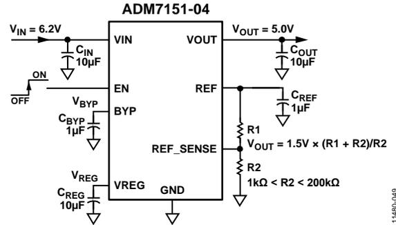
Figure 49. Typical Adjustable Output Voltage Application Schematic
