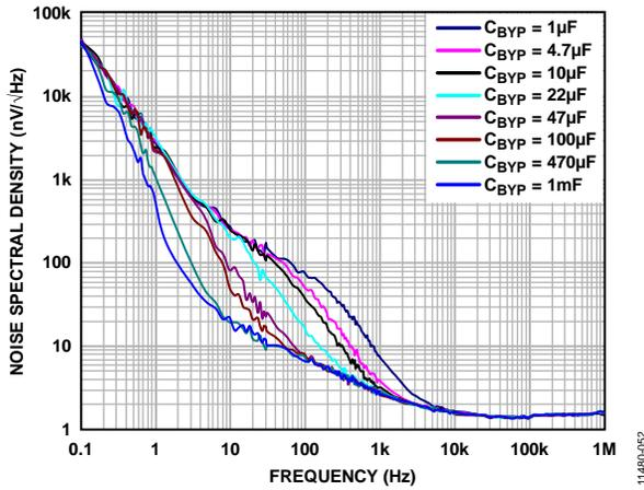
Figure 52. Noise Spectral Density vs. Frequency, C<sub>BYP</sub> = 1 μF to 1 mF
