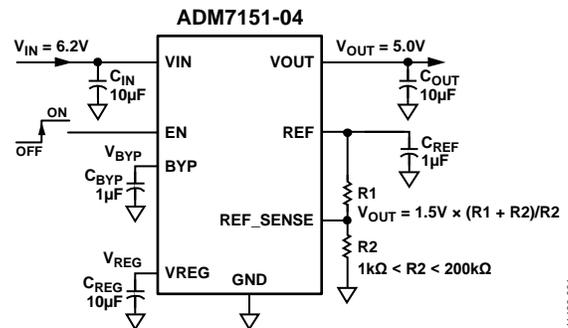
Figure 1. **ADM7151-04** with  $V_{\text{OUT}} = 5\text{ V}$
