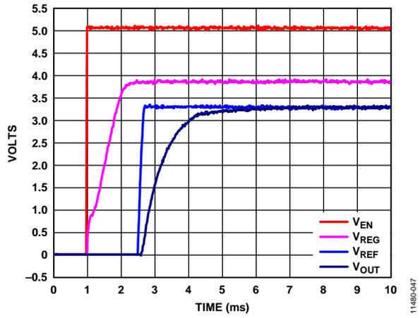
Figure 47. V<sub>OUT</sub>, V<sub>REF</sub>, V<sub>REG</sub> Start-Up Times After V<sub>EN</sub> Rising,
