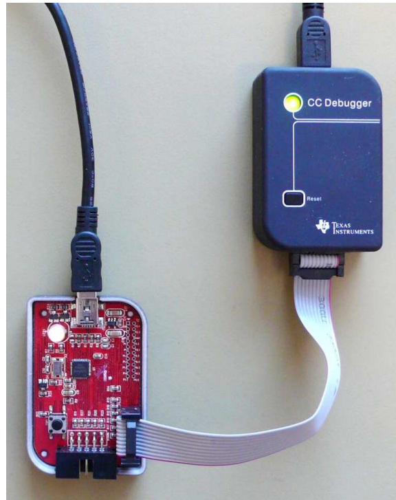
Figure 18. Programming the Bootloader on the CC Debugger Using Another CC Debugger
