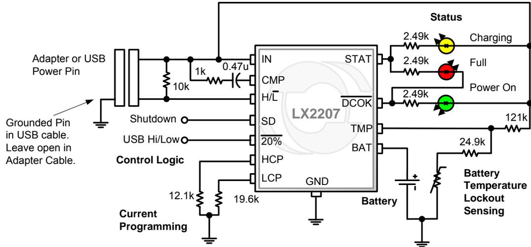
**Figure 1** – Typical Application – 750mA adapter charge current and 500mA or 100mA maximum USB charge currents. A grounded spare pin in the USB power cable can be used to sense when the 500mA USB current power source is being used. This application also uses three LED indicators for Power attached, Battery Charging and Battery full. This configuration also implements circuitry to lockout battery charging if the battery is less than 0C or greater than 60C.
