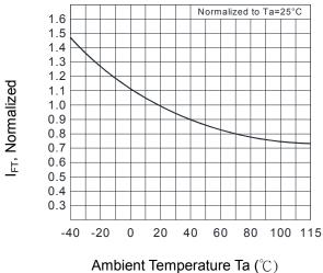
Fig.2 On-State R.M.S. Current vs. Ambient Temperature
