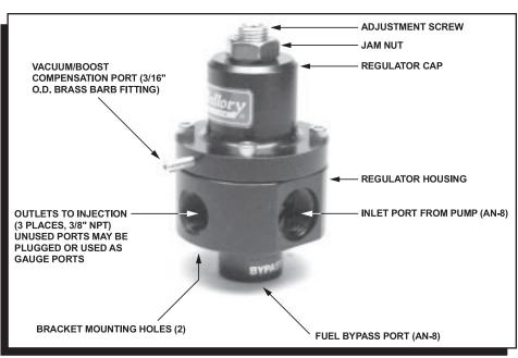
(vacuum compensation) at idle and part throttle, or increase fuel pressure under blower boost (boost compensa- tion). While it is not necessary to connect a hose to the vacuum/boost compensation port, it may be beneficial in some cases. However, the small plug on the barb must be removed before use.
