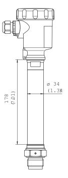
LBV320 with PUR suspension cable, threaded version G  $1\frac{1}{2}$  A (DIN ISO 228/1)
