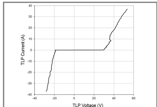
Fig.6 Transmission Line Pulsing (TLP) Measurement
