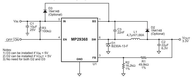
Figure 3—1.4MHz, 3.3V Output at 1A Step-Down Converter
