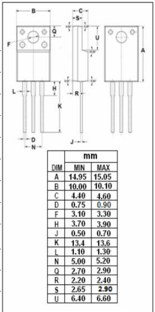
**isc N-Channel MOSFET Transistor TK20A60W5, ITK20A60W5**
