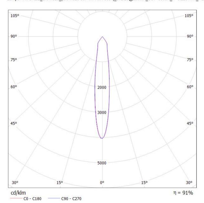
NOTE: The typical divergence will be changed by different color, chip size and chip position tolerance. The typical total divergence is the full angle measured where the luminous intensity is half of the peak value.
