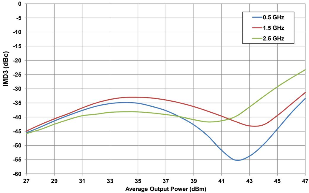
**Figure 4. - Third Order Intermodulation Distortion vs Frequency measured in Broadband Amplifier Circuit CGHV40100-AMP**
