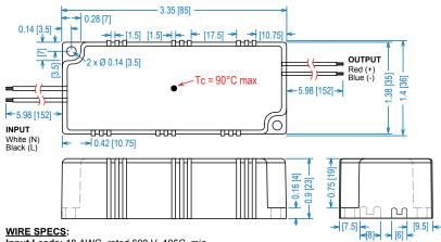
Input Leads: 18 AWG, rated 600 V, 105C, min. Output Leads: 18 AWG, rated 300 V, 105C, min. All wires are stranded with solder dipped ends.
