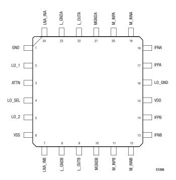
Figure 2. SKY42054 Pinout – 24-Pin PQFP Package (Top View)
