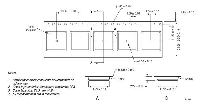
Figure 15. SKY42054 24-Pin PQFP Tape and Reel Dimensions
