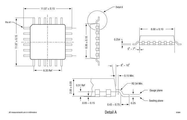
Figure 14. SKY42054 24-Pin PQFP Package Dimensions
