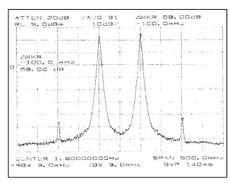
Figure 3. LNA (IIP3 = +19 dBm, Input Power = -15 dBm)
