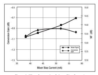
Figure 8. Mixer Conversion Gain vs Bias Current
