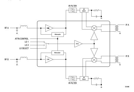
Figure 1. SKY42054 Functional Block Diagram
