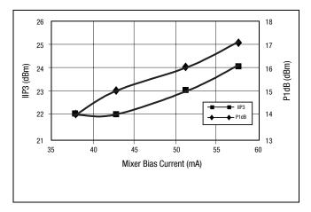
Figure 9. Mixer IIP3 and +1 dB Compression Point vs Bias Current
