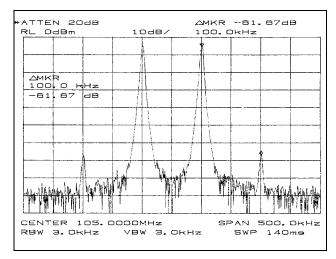
Figure 5. Mixer With Low Side L0 (IIP3 = +20 dBm, Input Power = -10 dBm)
