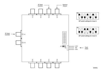
Figure 13. SKY42054 Evaluation Board Mixer Testing Configuration
