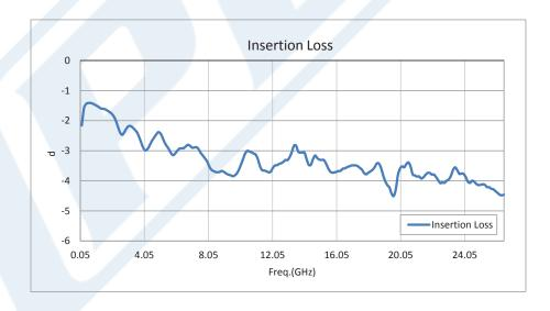
Click the following link (or enter part number in "SEARCH" on website) to obtain additional part information including price, inventory and certifications: SMA SPDT PIN Diode Switch Operating From 50 MHz to 26.5 GHz Up To +27 dBm PE71S2010
