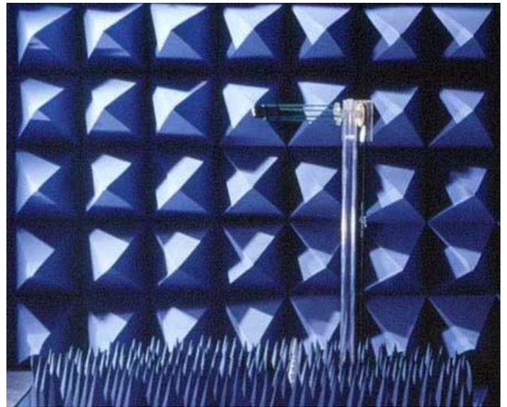
Antenna Setup in CTIA 3D Chamber
