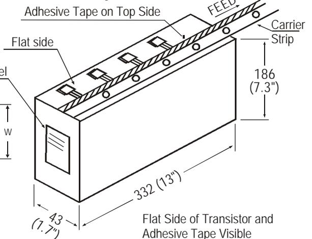
Flat Side of Transistor and Adhesive Tape Visible
