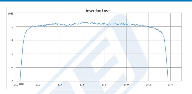
Click the following link (or enter part number in "SEARCH" on website) to obtain additional part information including price, inventory and certifications: 8 Section Bandpass Filter With SMA Female Connectors Operating From 17.3 GHz to 18.1 GHz With a 800 MHz Passband PE87FL1006
