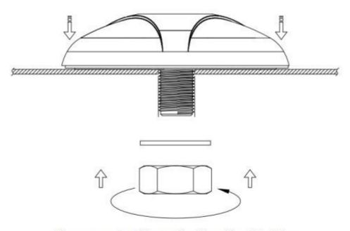
Recommended Torque for Mounting 29.4 N·m Maximum Torque for Mounting 39.2N·m
