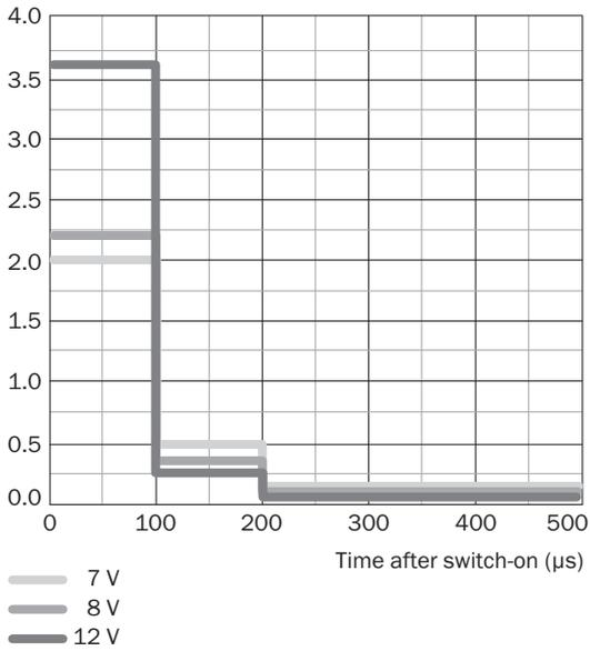
This diagram shows the switch-on current
