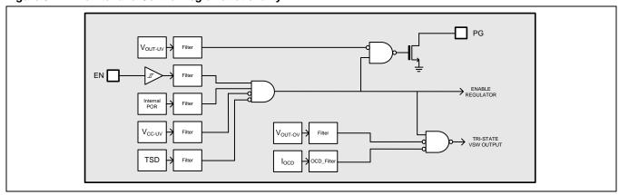
Figure 3.2 Monitor and Control Logic Functionality
