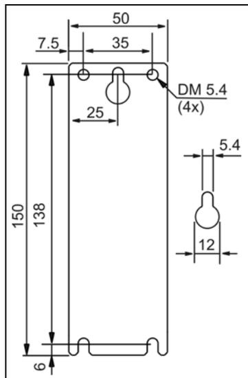
Fig. 24-6 **Wall/panel mounting, side view**
