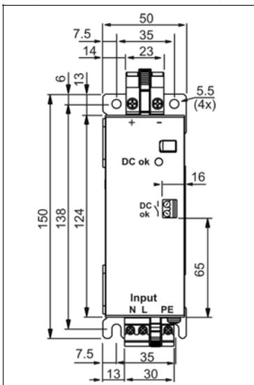
Fig. 24-5 **Hole pattern for wall mounting**
