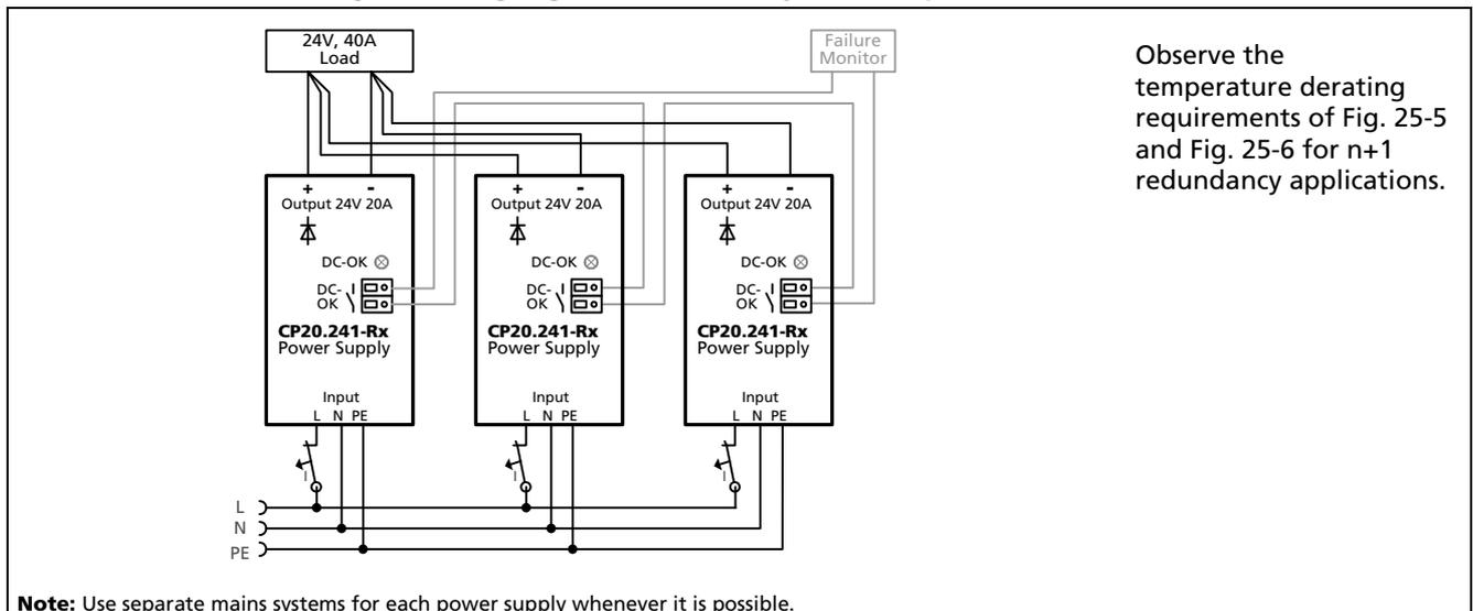
Observe the temperature derating requirements of Fig. 25-5 and Fig. 25-6 for n+1 redundancy applications.
