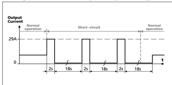
Fig. 6-3 Dynamic overcurrent capability, typ.
