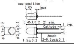
Figure-10 Ø 4Mold (Type 42)
