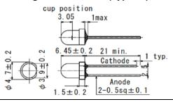
Figure-11 Ø 3Mold (Type 31)
