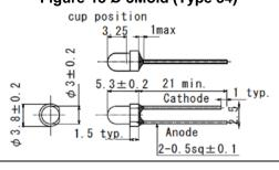
Figure-14 Ø 3Mold (Type 36)
