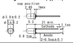
Figure-13 Ø 3Mold (Type 34)
