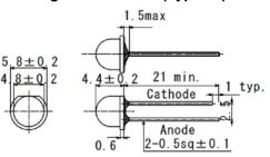
Figure-9 Ø 4Mold (Type 41)
