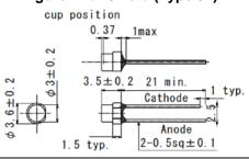
Figure-12 Ø 3Mold (Type 33)
