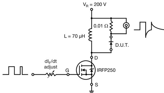
Fig. 9 - Reverse Recovery Parameter Test Circuit
