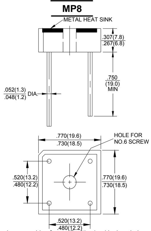
Polarity shown on side of case, Positive lead by beveled corner.
