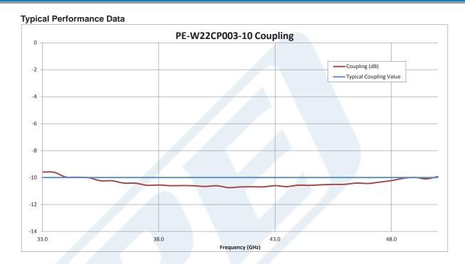
Click the following link (or enter part number in "SEARCH" on website) to obtain additional part information including price, inventory and certifications: WR-22 10 dB Directional Waveguide Coupler With UG-383/U Flange and E-Plane Coupled Port From 33 GHz to 50 GHz Q Band PE-W22CP003-10
