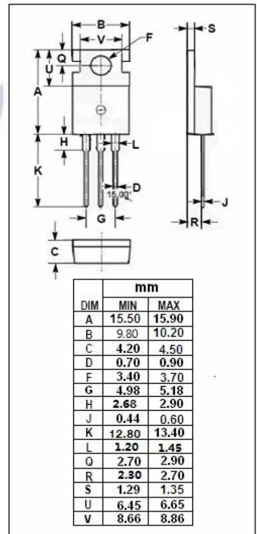
**isc Three Terminal Positive Voltage Regulator****L7805CV****• ELECTRICAL CHARACTERISTICS**
