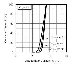
Figure 7. Transfer Characteristics
