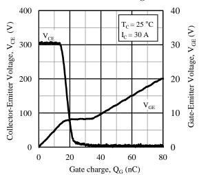
Figure 12. Gate Charge Characteristics
