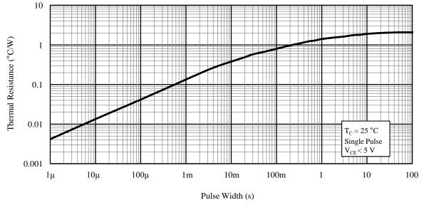
Figure 17. Transient Thermal Resistance
