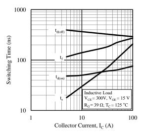
Figure 16. Switching Time vs. Collector Current
