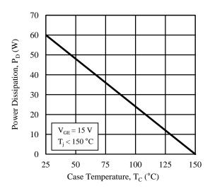
Figure 3. Power Dissipation vs. Case Temperature
