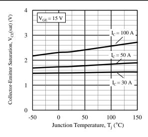
Figure 8. Saturation Voltage vs. Junction Temperature
