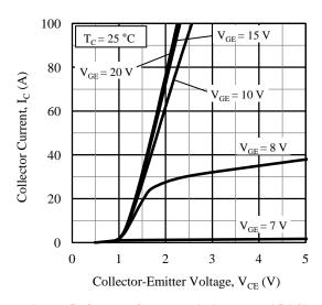
Figure 5. Output Characteristics ( $T_C = 25$  °C)
