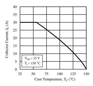
Figure 4. Collector Current vs. Case Temperature
