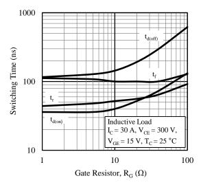
Figure 13. Switching Time vs. Gate Resistor
