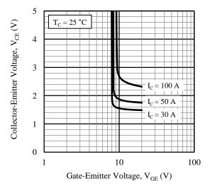
Figure 9. Collector-Emitter Voltage vs. Gate-Emitter Voltage
