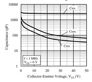
Figure 11. Capacitance Characteristics
