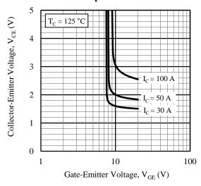
Figure 10. Collector-Emitter Voltage vs. Gate-Emitter Voltage
