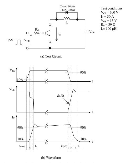
Figure 1 Test Circuits and waveforms of dv/dt and Switching Time
