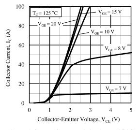
Figure 6. Output Characteristics ( $T_C = 125$  °C)
