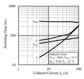
Figure 15. Switching Time vs. Collector Current
