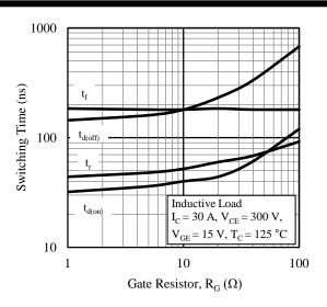
Figure 14. Switching Time vs. Gate Resistor
