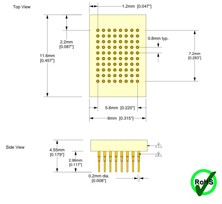
Substrate: 1.59mm ±0.18mm [0.0625" ±0.007"] FR4/G10 or equivalent high temp material; Non-clad
