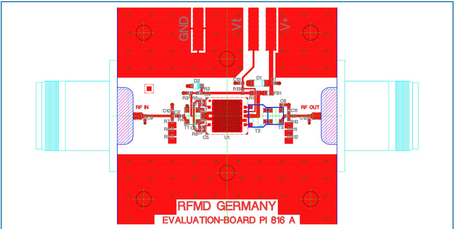
Note: The ground plane of the RFCM3326 module should be soldered onto a board equipped with as many thermal vias as possible. Underneath this thermal via array a heat sink with thermal grease needs to be placed which is able to dissipate the complete module DC power (up to 10.4 Watts). In any case the module backside temperature should not exceed 110°C.
