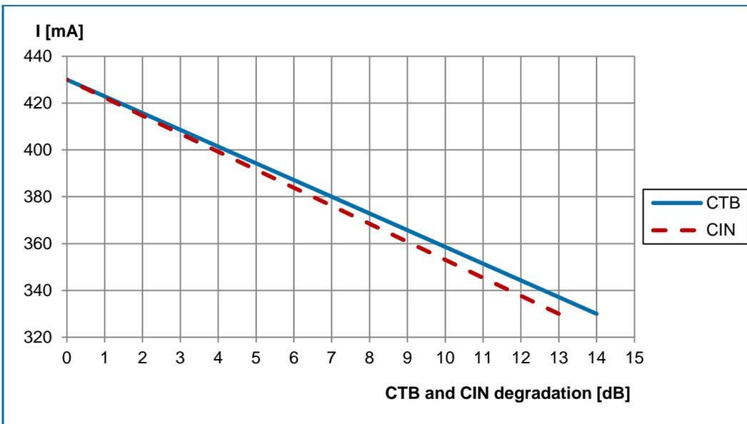
**Test condition:** V+= 24V; T<sub>MB</sub>=30°C; Z<sub>S</sub>=Z<sub>L</sub>=75Ω; V<sub>O</sub>=61dBmV at 1000MHz, 18dB extrapolated tilt, 79 analog channels plus 75 digital channels (-6dB offset)
