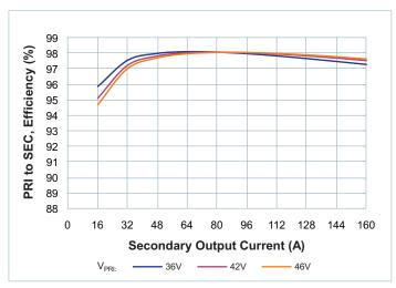
**Figure 10** — Efficiency at  $T_{CASE} = 80^{\circ}C$
