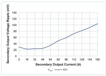
**Figure 13** — V<sub>SEC\_OUT\_PP</sub> vs. I<sub>SEC\_DC</sub>; No external C<sub>SEC\_OUT\_EXT.</sub> Board mounted module, scope setting: 20MHz analog BW
