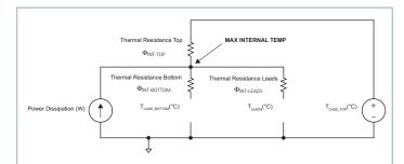
Figure 24 — Top case thermal model
