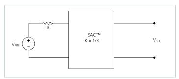
**Figure 20** — K = 1/3 Sine Amplitude Converter with series primary resistor
