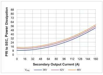
**Figure 11** — Power dissipation at  $T_{CASE} = 80$ °C
