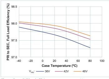
**Figure 5** — Full load efficiency vs. temperature;  $V_{PRI\_DC}$
