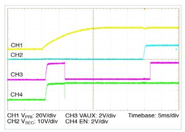
**Figure 17** — Start up from application of  $V_{PRI\_DC}$ = 42V, 20%  $I_{SEC\_DG}$  100%  $C_{SEC\_DUT\_EXT}$
