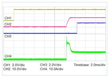
**Figure 18** — Start up from application of EN with pre-applied  $V_{PRI\_DC} = 42V$ , 20%  $I_{SEC\_DC}$ , 100%  $C_{SEC\_OUT\_EXT}$
