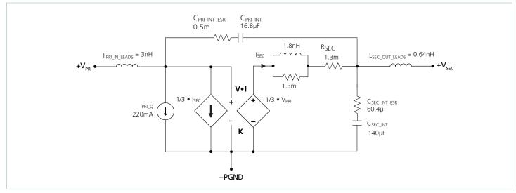
Figure 19 — NBM module AC model
