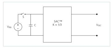
**Figure 21** — Sine Amplitude Converter with primary capacitor
