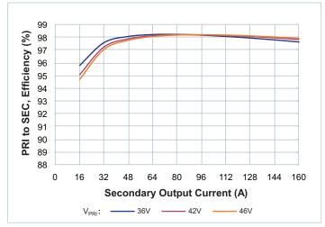
**Figure 8** — Efficiency at  $T_{CASE} = 25^{\circ}C$
