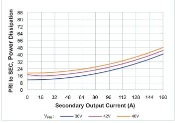
**Figure 7** — Power dissipation at  $T_{CASE} = -40$ °C
