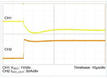
**Figure 15** — 0A - 160A transient response:  $C_{PRI\_IN\_EXT} = 270\mu F$ , no external  $C_{SEC\_OUT\_EXT}$
