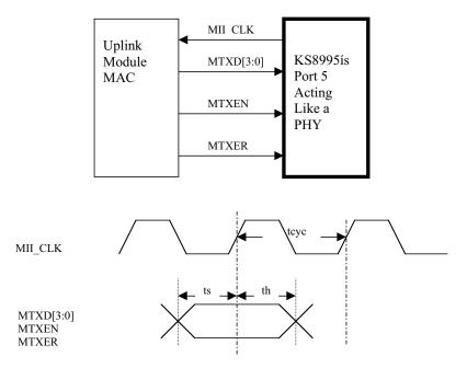
Figure 6. Reverse MII Timing-Receive Data from MII
