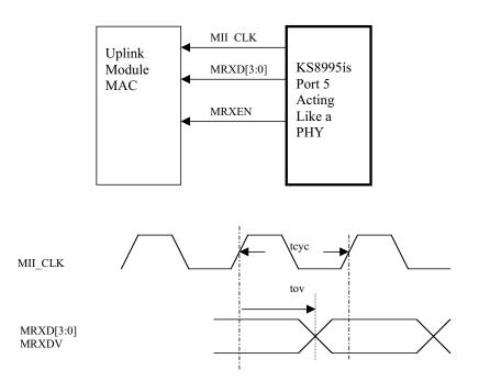
Figure 7. Reverse MII Timing-Transmit Data to MII
