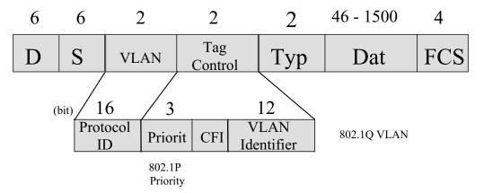
Figure 10. 802.1q and 802.1p Frame Format
