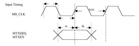
Figure 4. SNI (7-Wire) Input Timing
