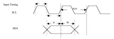
Figure 2. EEPROM Input Timing
