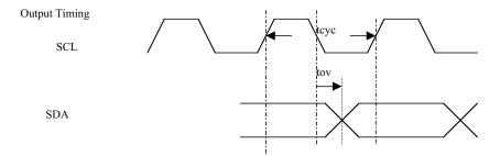
Figure 3. EEPROM Output Timing
