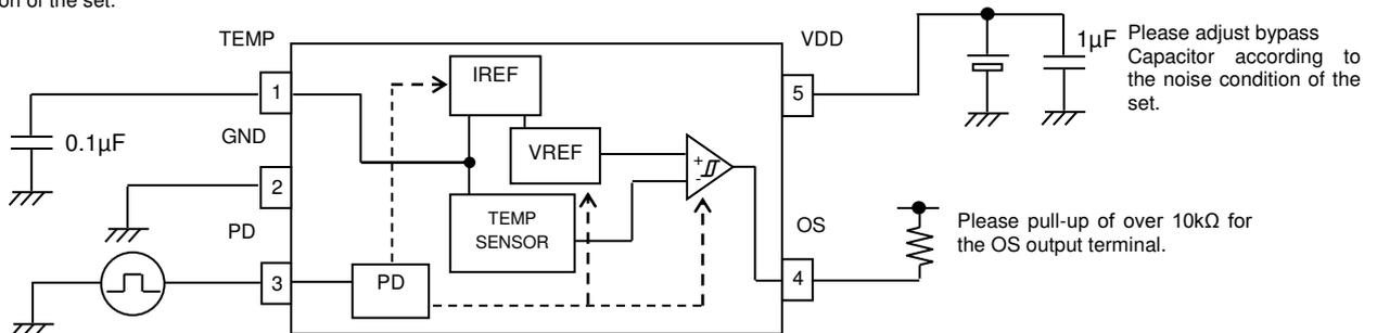
Block Diagram and Pin Configuration
