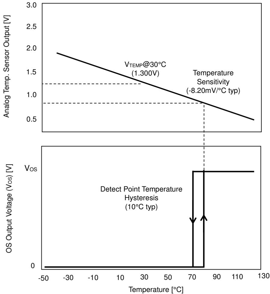
If the temperature exceeds the detect point temperature, the internal comparator forces the OS output to change from “L” to “H”. (ex. Active-H Type)
