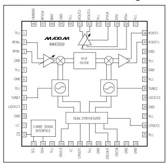
Pin Configurations/Functional Diagrams continued at end of data sheet.
