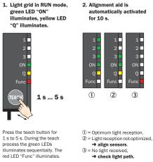
3. Light grid in RUN mode, green LED "ON" illuminates, yellow LED "Q" illuminates.
