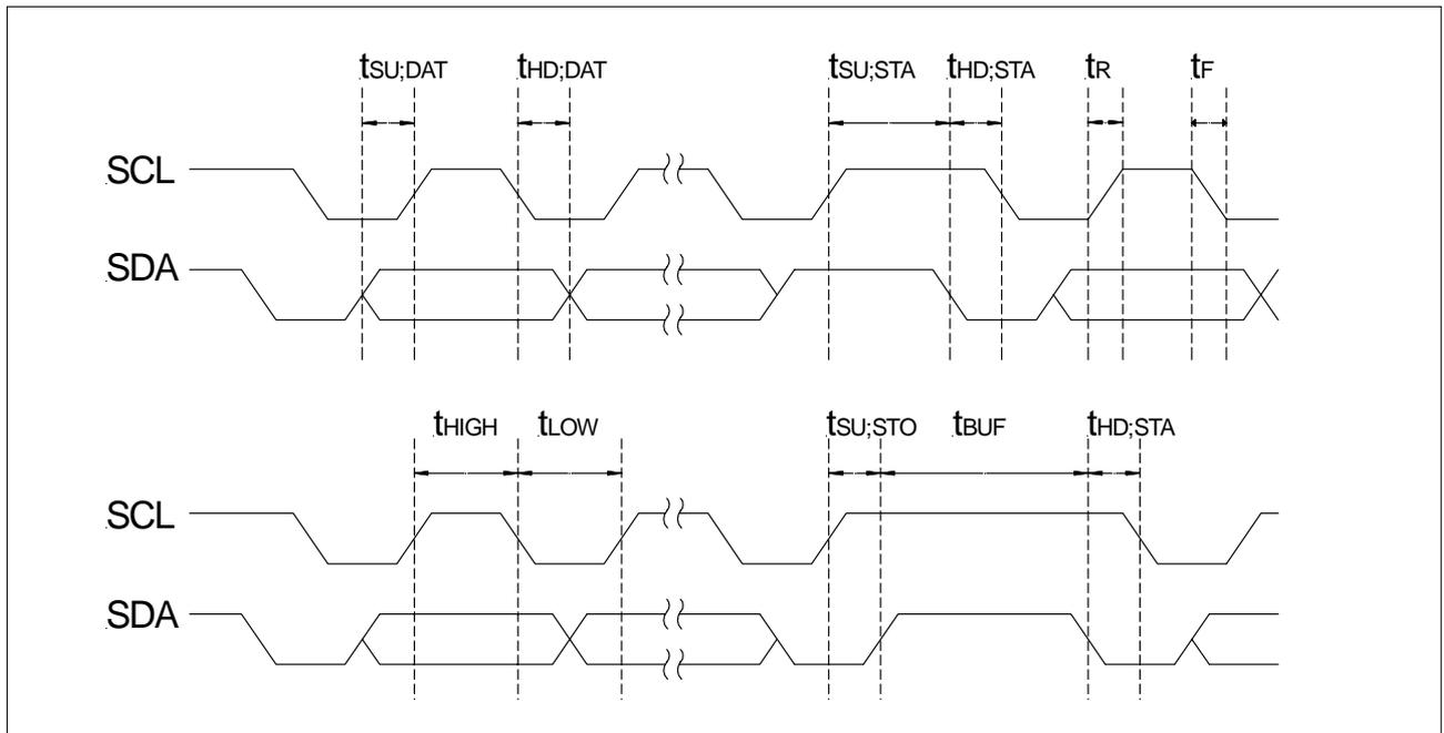
Fig. 2: Timing characteristics
