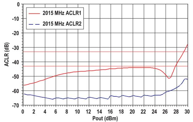
Figure 10. ACLR vs. Pout at 2015 MHz.
