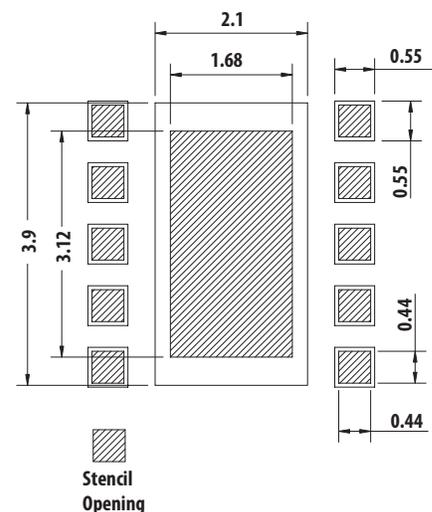
Figure 5. Combined PCB and stencil layouts
