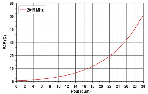
Figure 11. PAE vs. Pout at 2015 MHz.
