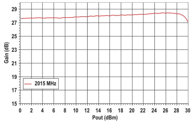
Figure 12. Gain vs. Pout at 2015 MHz.
