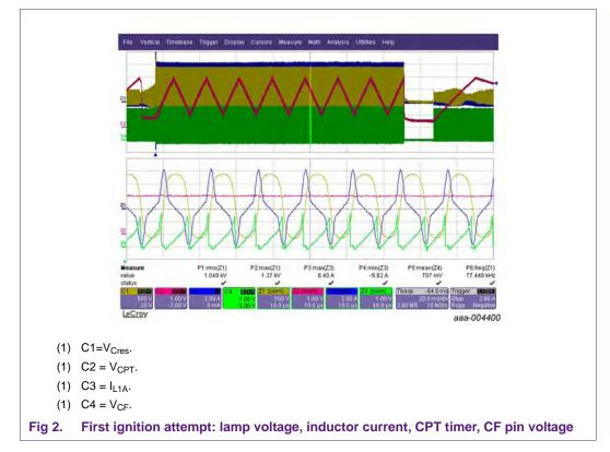
Figure 2 shows the fault timer counting on channel C2. The VFB pin activates counting and is necessary to shut down the ballast in case no lamp is present.
