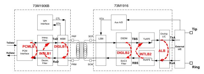
Figure 39: Loopback Modes Highlighted
