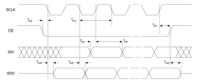
Figure 7: SPI Timing Diagram
