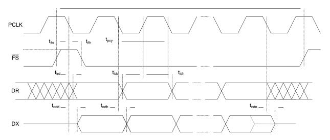
Figure 9: PCM Timing Diagram for Negative Edge Transmit Mode and Positive Edge Receive Mode
