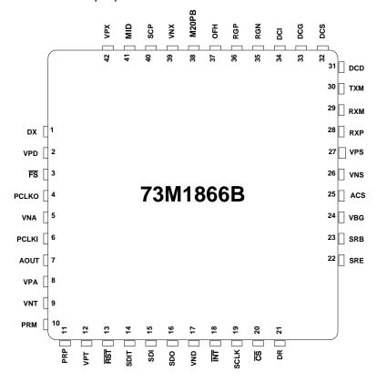
Figure 6: 73M1866B 42-Pin Pinout
