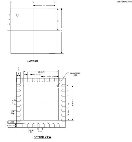
Figure 48: 32-Pin QFN Package Dimensions
