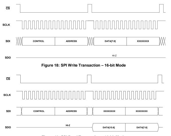
Figure 19: SPI Read Transaction - 16-bit Mode
