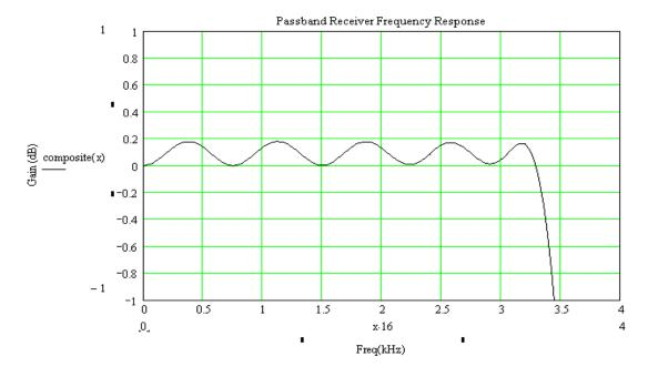
Figure 30: Pass-band Response of the Overall Receive Path
