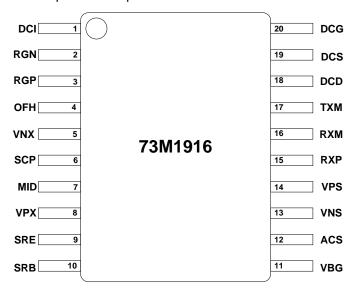
Figure 3: 73M1916 20-Pin TSSOP Pinout
