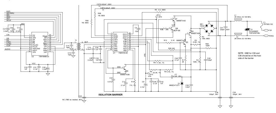
Figure 12: Recommended Circuit for the 73M1966B
