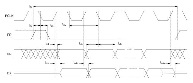
Figure 8: PCM Timing Diagram for Positive Edge Transmit Mode and Negative Edge Receive Mode
