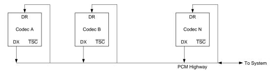
Figure 22: Example of PCM Highway Interconnect
