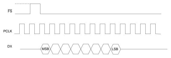
Figure 20: 8-bit Transmission Example
