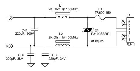
Figure 14: Suggested Over-Voltage Protection and EMI Suppression Circuit
