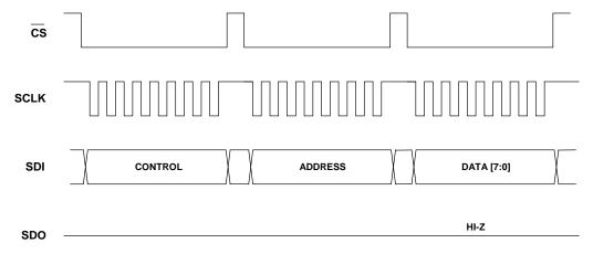
Figure 16: SPI Write Operation – 8-bit Mode
