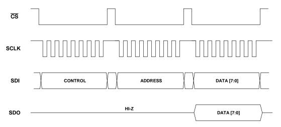
Figure 17: SPI Read Transaction - 8-bit Mode
