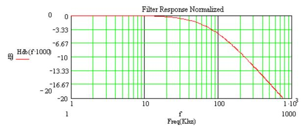
Figure 10: Frequency Response of the Call Progress Monitor Filter
