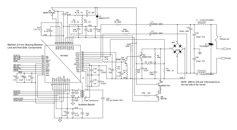
Figure 13: Recommended Circuit for the 73M1866B
