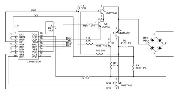
Figure 32: Line-Side Device AC and DC Circuits
