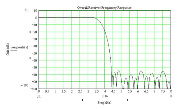
Figure 29: Overall Frequency Response of the Receive Path
