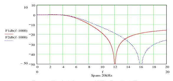
Figure 37: Magnitude Response of Billing Tone Notch Filter
