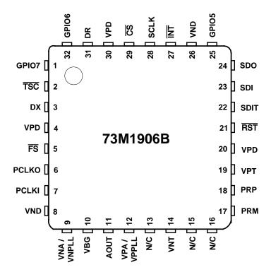
Figure 4: 73M1906B 32-Pin QFN Pinout
