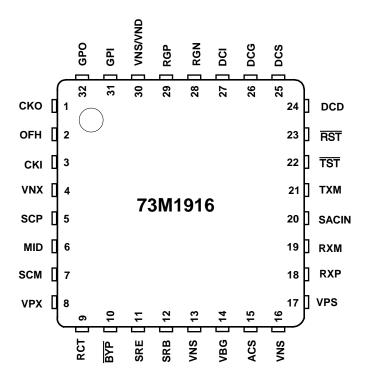
Figure 5: 73M1916 32-Pin QFN Pinout
