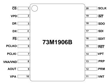
Figure 2: 73M1906B 20-Pin TSSOP Pinout
