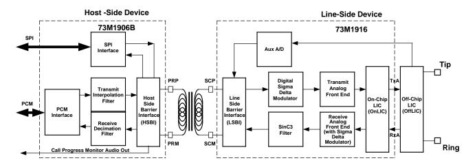
Figure 1: Simple 73M1x66B Reference Block Diagram
