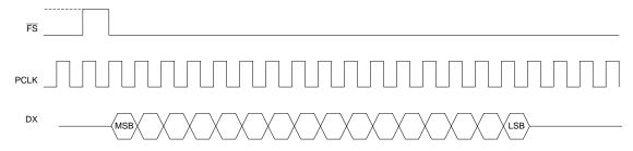
Figure 21: 16-bit Transmission Example
