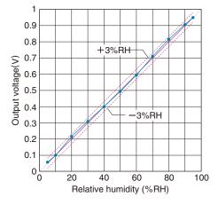
Example of thermal characteristics(Temperature dependency) at Edc=5V, +5 to +45°C, 5% to 95%RH
