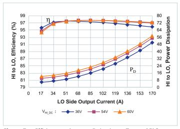
**Figure 7** — Efficiency and power dissipation at  $T_{CASE} = 25$ °C
