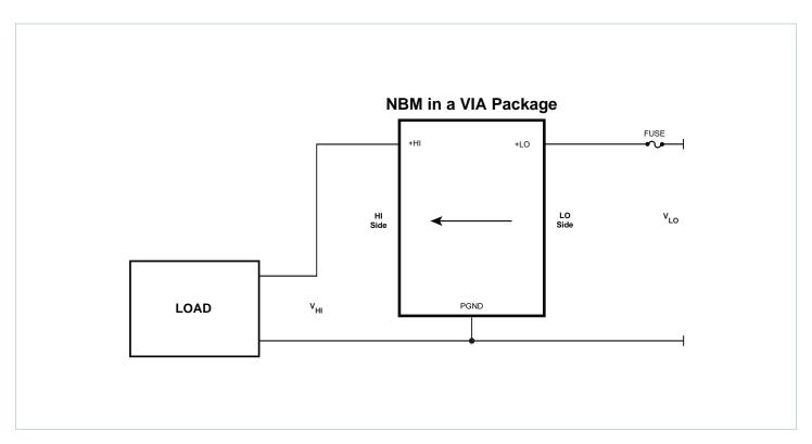
NBM3814x60E12A7yzz providing fixed ratio step-up DC-DC conversion. NBM is operating in reverse direction.
