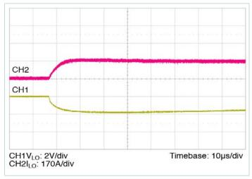
**Figure 12** — 0A– 170A transient response:  $C_{HL\,IN\_EXT} = 300\mu F$ , no external  $C_{LO\_OUT\_EXT}$
