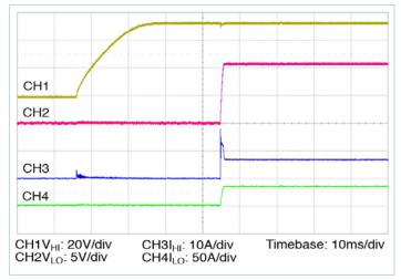
**Figure 14** — Forward start up from application of  $V_{HLDC}$  = 54V, 20%  $I_{LO\ DC}$ , 100%  $C_{LO\ OUT\ EXT}$
