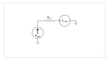
**Figure 20** — Single-sided cooling VIA thermal model
