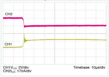
**Figure 13** — 170A – 0A transient response:  $C_{HI\_IN\_EXT} = 300\mu F$ , no external  $C_{LO\_OUT\_EXT}$
