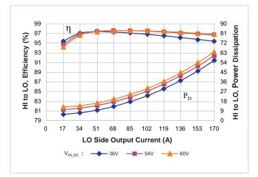
**Figure 8** — Efficiency and power dissipation at  $T_{CASE} = 85^{\circ}C$
