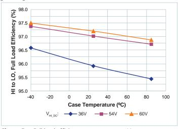
**Figure 5** — Full load efficiency vs. temperature;  $V_{HI\_DC}$
