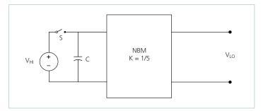
Figure 18 — NBM with HI side capacitor
