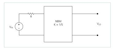
**Figure 17** — K = 1/5 NBM with series HI side resistor
