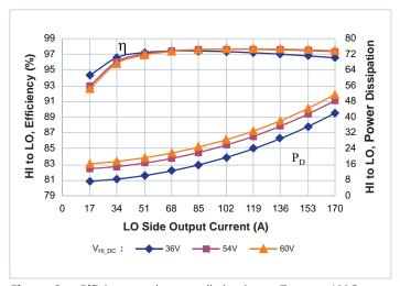
**Figure 6** — Efficiency and power dissipation at  $T_{CASE} = -40$ °C
