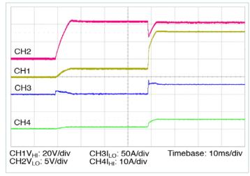
Figure 15 — Reverse start up from application of  $V_{LO\_DC} = 10.8V$ , 20%  $I_{HI\_DC}$ , 100%  $C_{HI\_OUT\_EXT}$
