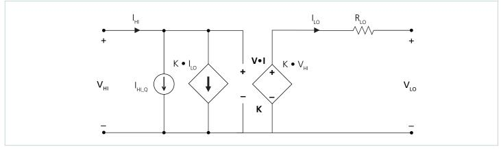
Figure 16 — NBM DC model (Forward direction)
