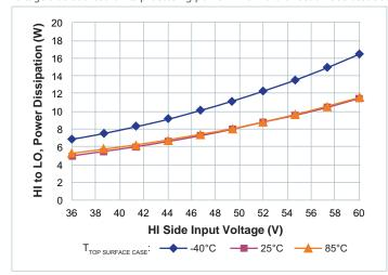
Figure 4 — No load power dissipation vs. V<sub>HI DC</sub>
