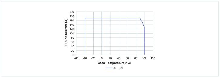
**Figure 1** — Specified thermal operating area
