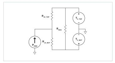
Figure 19 — Double sided cooling VIA thermal model
