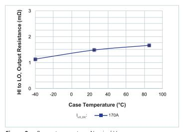
**Figure 9** —  $R_{LO}$  vs. temperature; Nominal  $V_{HI\_DC}$   $I_{LO}$   $D_{C} = 170A$  at  $T_{CASE} = 85^{\circ}C$
