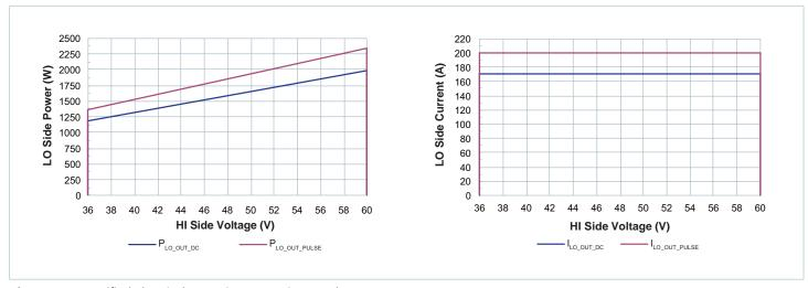
Figure 2 — Specified electrical operating area using rated R<sub>LO\_HOT</sub>
