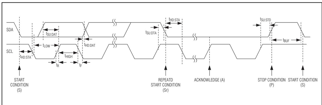
Figure 2. I<sup>2</sup>C Serial-Interface Timing Diagram
