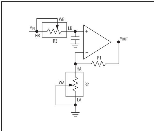
Figure 15. Programmable Filter
