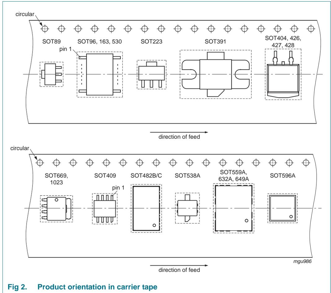
Fig 2. Product orientation in carrier tape
