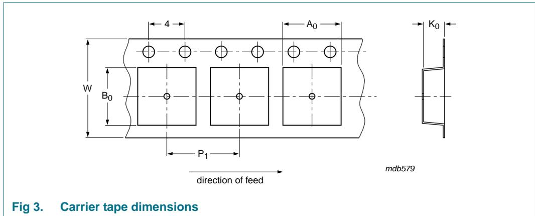
**Fig 3. Carrier tape dimensions**
