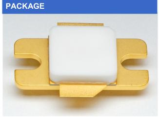
The device utilizes a RoHS compliant metal ceramic flanged package with a ceramic lid. The HV400A package style is qualified for gross leak test – MIL-STD-883, Method 1014.
