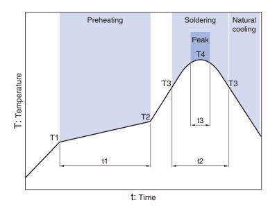
Soldering Preheating Peak Temp. Temp. Time Time Temp. Time T1 **T2 T**4 t1 тз t2 t3 150°C 180°C 60 to 120s 230°C 250°C 30s 5s
